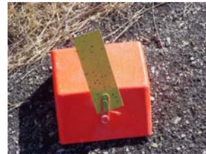
Water sensitive card used to sample spray droplets
