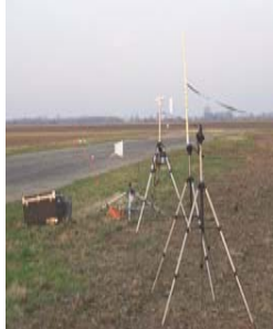
Flight-line equipment used to measure spray pattern
