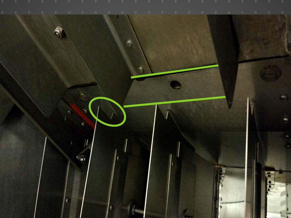
These gaps must be sealed to prevent material from bypassing spreader Use two layers of engine baffle material to fill these gaps
