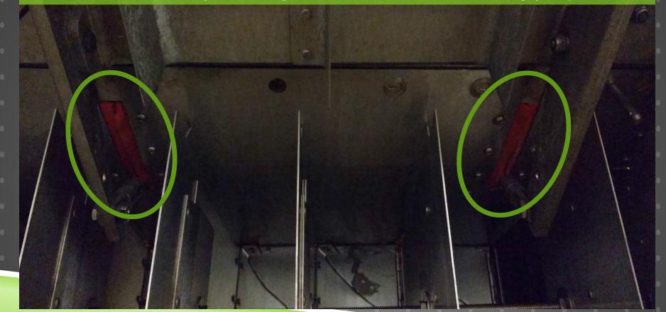
Angle between top of spreader and bottom of wing root must be between 0 – 1 degree spreader tail down
