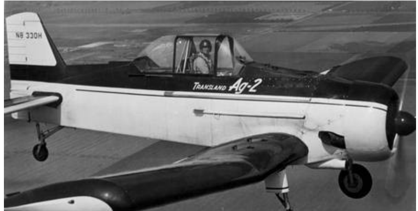
The designers of Transland's Ag-2 emphasized greater payload and a design that could be produced in volume. Airframe construction began in 1954.
