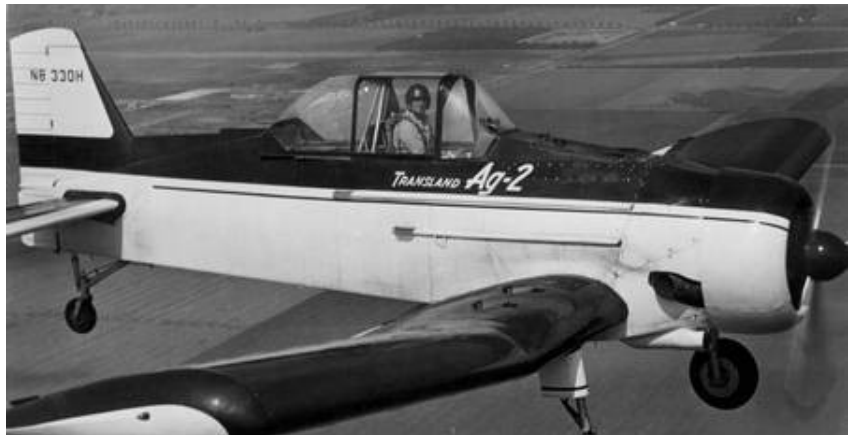
The designers of Transland's Ag-2 emphasized greater payload and a design that could be produced in volume. Airframe construction began in 1954.
